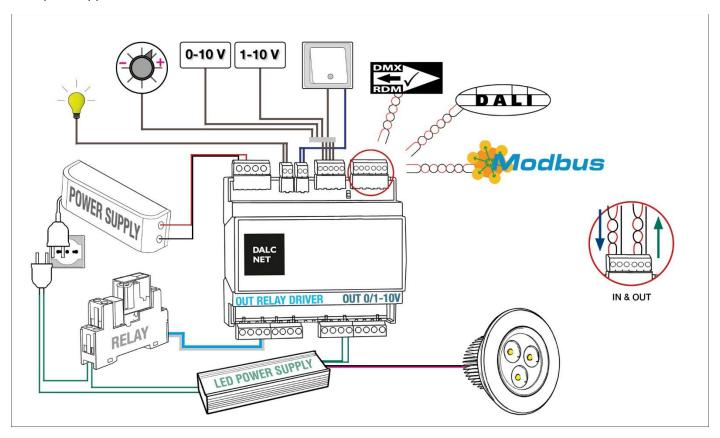
Thanks to DIM CONVERTER is possible to command the power supplies with DIM Function (with 0/1-10V command) to dim the load connected to it
